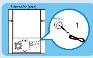
Connect the FM antenna to the inner pin of the 0 FM 75  $\Omega$  socket (for some models, this cable has been connected). Extend the antenna for optimum reception.
