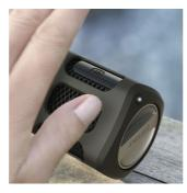
SHOQBOX is equipped with a motion sensor. Simply swipe over the sensor from left to right or right to left, to skip to the next or last track. Put your hand over the sensor for a second to pause the music. Do it again to put it back on. Easy gesture control allows you to control your music the simplest way.
