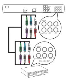
Connect the 5.1-channel audio cables (not supplied) to the 5.1CH AUDIO OUTPUT sockets on this player and the corresponding AUDIO input sockets on the device.
