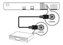
1 Connect a coaxial cable (not supplied) to the COAXIAL socket on this player and the COAXIAL/DIGITAL input socket on the device.
