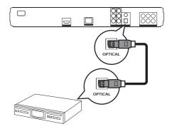
1 Connect an optical cable (not supplied) to the OPTICAL socket on this player and the OPTICAL/DIGITAL input socket on the device.
