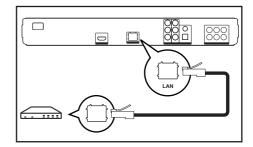
Connect the network cable (not supplied) to the LAN socket on this player and the LAN socket on the broadband modem or router.
