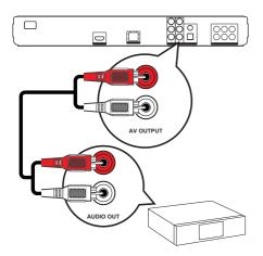
Connect the audio cable to the AUDIO L/R-AV OUTPUT sockets on this player and the AUDIO input sockets on the device.
