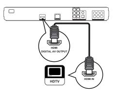
1 Connect an HDMI cable to the HDMI socket on this player and the HDMI input socket on the TV.
