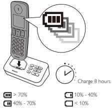
Flashing: low battery Scrolling: charging in progress
