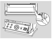
Insert the USB device's USB plug into the socket on the set 's foldable control panel.
