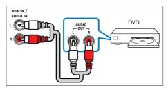
1 Using an analog cable, connect the AUX connectors on this product to the AUDIO OUT connectors on the TV or other device.
