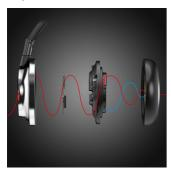
Fidelio NC-1 uses a feed-forward and feed-backward active noise cancellation (ANC) solution, which means there are 4 microphones implemented inside and outside the ear cans to capture noise for advanced processing. The feed-forward ANC (mic outside the ear can) covers a wider bandwidth of frequencies, while the feed-backward ANC
