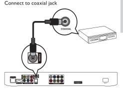
1 Connect a coaxial cable (not supplied) to:
