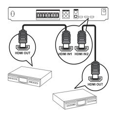
1 Connect an HDMI cable (not supplied) to the HDMI IN1/HDMI IN2 socket on the Digital Receiver and the HDMI OUT socket on the device
