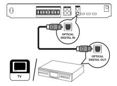
1 Connect the optical cable to the OPTICAL DIGITAL-IN socket on the Digital Receiver and the OPTICAL/SPDIF output socket on the device.
