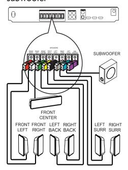
1 Connect the speakers and subwoofer to the matching sockets on the Digital Receiver.
