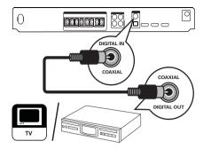
1 Connect a coaxial cable (not supplied) to the COAXIAL DIGITAL-IN socket on the Digital Receiver and the COAXIAL/ DIGITAL output socket on the device.
