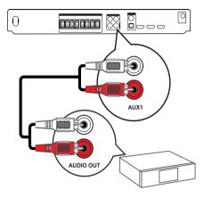
1 Connect the audio cables (not supplied) to the AUDIO IN-AUX1 sockets on the Digital Receiver and the AUDIO output sockets on the device.
