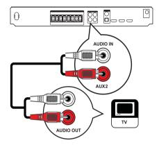
1 Connect the audio cable (not supplied) to the AUDIO IN-AUX2 sockets on the Digital Receiver and the AUDIO OUT sockets on your TV.
