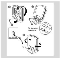
Position the antenna as far as possible from a TV, VCR or other radiation source.
