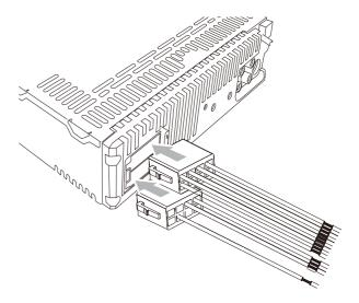
Check the car's wiring carefully and connect them to the supplied male connector.
