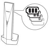
Charge your handset by docking it in either direction. When the handset is placed correctly on the base station, you hear a docking tone (see 'Set the docking tone' on page 23). The LED at the
