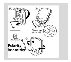
Position the antenna as far as possible from a TV, VCR or other radiation source.
