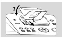
To connect with a different iPod portable player, pop up the corresponding dock adapter and replace with a new one of the matching type.
