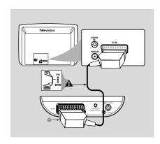
Use the SCART cable (black) to connect the DVD Player's SCART jack (SCART) to the corresponding Scart input jacks on the TV.
