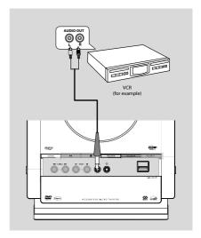
Connect the system's AUX-IN jack to the AUDIO OUT jacks on another audio/visual device (such as a VCR, Laser Disc player or cassette desk) using a "single-to-double" cinch cable (with one end providing a 3.5" connector for connection to the AUX-IN jack while the other end providing two white/red connectors for connection to the other device's AUDIO OUT jacks).
