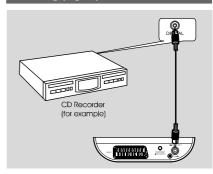
Connect the **COAXIAL** (**DIGITAL OUTPUT**) jack on the video box to the
