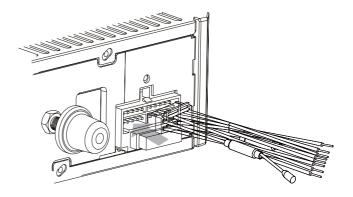
2 Connect the other end of the supplied standard connector to the unit.
