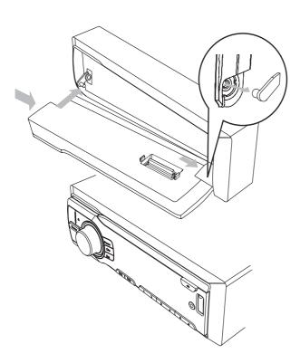
2 Insert the right side of the panel in the chassis until it is correctly engaged.
