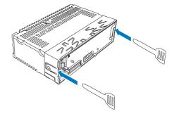
Install the sleeve into the dashboard and bend the tabs outward to fix the sleeve.
