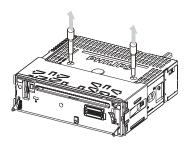
Remove the mounting sleeve with the supplied disassembly tools.
