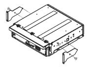
**4** Place the supplied rubber cushion over the end of the mounting bolt.
