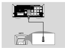
Use a HDMI cable (not supplied) to connect the HDMI jack on the DVD Player to HDMI IN on a HDMI compatible device (e.g.; TV, Projector; Adaptor).
