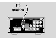
Connect the supplied FM antenna to the FM ANTENNA (75 Ω) jack. Extend the FM antenna and fix its end to the wall.
