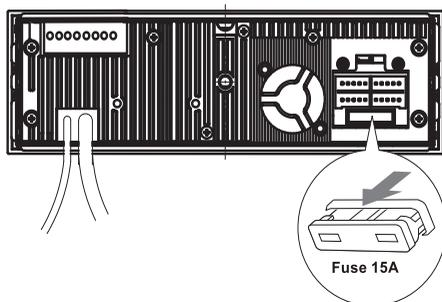
If the fuse gets damaged immediately after it has been replaced, there may be an internal malfunction. In such case, consult your Philips dealer.
