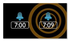
To counter oversleeping, the Philips Clock radio has a snooze feature. Should the alarm ring and you wish to continue sleeping a bit longer, simply press the Repeat Alarm button once and go back to sleep. Nine minutes later the alarm will ring again. You can continue to press the Repeat Alarm button every nine minutes until you turn off the alarm altogether.
