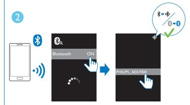
Enable Bluetooth®, then select 'PHILIPS\_AEA7000' on your mobile device (if necessary, input '0000' as the paring password).
