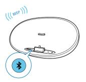
Next time you switch on DS3480, the speaker connects to the last paired device automatically.
