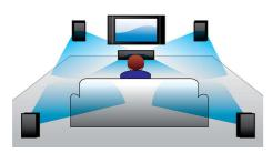
A built-in Dolby Digital decoder eliminates the need for an external decoder by processing all six channels of audio information to provide a surround sound experience and an astoundingly natural sense of ambience and dynamic realism. Dolby Pro Logic II provides five channels of surround processing from any stereo source.
