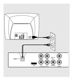
After everything is connected properly, plug in the AC power cord to the power outlet.
