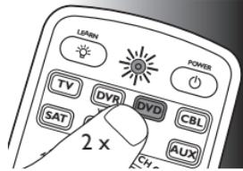
Press the device selection button **twice** to select the DVR part of the combo.
