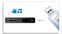
The Universal Serial Bus or USB is a protocol standard that is conveniently used to link PCs, peripherals and consumer electronic equuipment. Hi-Speed USB devices have a data transfer rate of up to 480 Mbps - up from the 12 Mbps in original USB ones. With Hi-Speed USB 2.0 Link, all you have to do is plug in your
