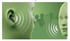
For face-to-face conversations, these earbuds can help you hear the other person better! Simply press the left earbud to activate Conversation Hearing mode or use the Philips Headphones app. Beamforming mics pick up the voice of the person in front of you while noise cancelling filters out ambient sounds.
