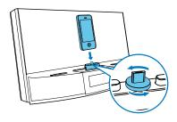
Adjust the bumpers on both sides of the connector to stabilize the phone.
