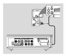
Use the SCART cable (black) to connect the DVD Player's SCART jack to the corresponding Scart input jacks on the TV (cable not supplied).
