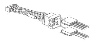
2 Connect the other end of the supplied standard connector to the unit.
