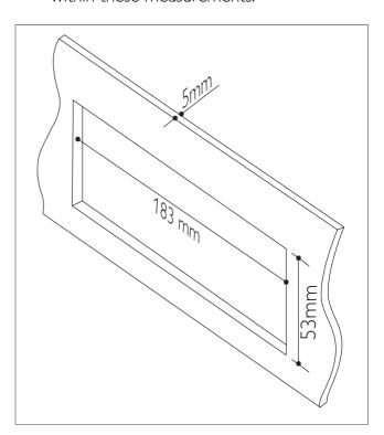
Install the sleeve into the dashboard and bend the tabs outward to fix the sleeve.
