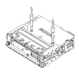
Remove the mounting sleeve with the supplied disassembly tools.
