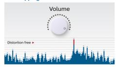
Anti-Clipping lets you play music louder and keeps it high quality, even when the battery is low. It accepts a range of input signals, from 300mV to 1000mV and keeps your speakers safe from damage by distortion. This built-in function monitors the musical signal as it goes through the amplifier and keeps peaks within the amplifier's range, preventing the audio distortion caused by clipping without affecting loudness. A
