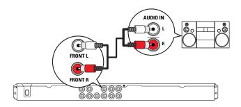
Connect the audio cables (supplied) to the AUDIO OUT FRONT L/R jacks on this DVD player and the audio input jacks on the device.
