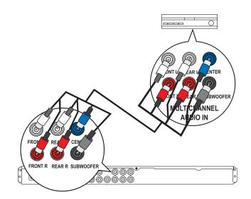
1 Connect the audio cables (not supplied) to the AUDIO OUT (FRONT L/R, REAR L/R, CENTER and SUBWOOFER) jacks on this DVD player and the audio input jacks on the device.
