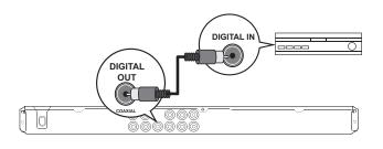
Connect a coaxial cable (not supplied) to the COAXIAL/DIGITAL OUT jack on this DVD player and the COAXIAL/DIGITAL input jack on the device.
