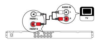
1 Connect the audio cables (supplied) to the AUDIO OUT FRONT L/R jacks on this DVD player and the audio input jacks on the TV.
