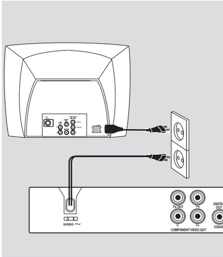
**After everything is connected properly, plug in the AC power cord to the power outlet.**
