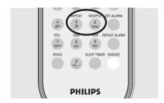
To return to normal playback, press REPEAT or/and SHUFFLE repeatedly until the various modes are no longer displayed
