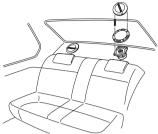
You can also mount the speakers into the surface of the rear tray.
