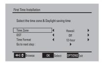
3 Select the time zone, DST and timer format, then press ▼ to select [Go to next step:] and press OK to confirm.
