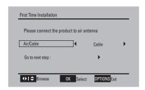
4 Select the antenna type as [Air], then press ▼ to select [Go to next step:] and press OK to confirm.
