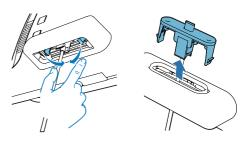
2 Release the inner locks and detach the cable from the docking adapter.
