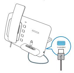
1 Lead the USB cable through the table stand and the hole in the dock, then connect it to the matching docking adapter.
