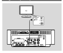
To listen to TV channels through this system, use the audio cables (white/red, not supplied) to connect AUX IN1 (L/R) jacks to the HEADPHONE jacks on the TV set (with a 3.5mm-diameter stereo jack).
