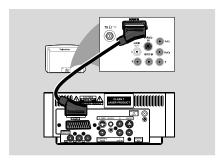
To listen to TV channels through this system, use the scart cable (not supplied) to connect the system's SCART jack to the corresponding SCART output jack on the TV set.
