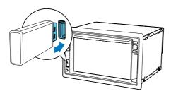
To remove the USB storage device, switch the system to another source first.
