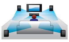
A built-in DTS and Dolby Digital decoder eliminates the need for an external decoder by processing all six channels of audio information to provide a surround sound experience and an astoundingly natural sense of ambience and dynamic realism. Dolby Pro Logic II provides five channels of surround processing from any stereo source.
