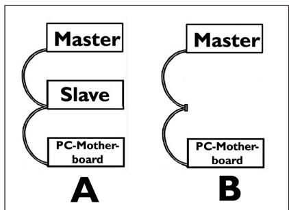
**UK** Connect the IDE cable like in A (2 devices) or B (only 1 device).
