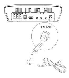
1 Connect the supplied FM antenna to the "FM ANT" socket on the unit.
