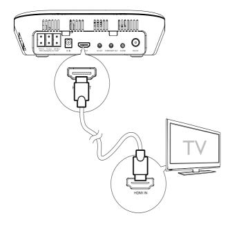
Connect HDMI (High Definition Multimedia Interface), DVI (Digital Visual Interface), or HDCP (High-bandwidth Digital Contents Protection)-compliant TVs through HDMI for the best picture quality. This connection transmits both video and audio signals. Through this connection, you can watch DVDs that contain HD (High-Definition) content.
