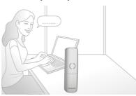
Handsfree mode uses a built-in loud speaker to amplify the voice of the caller, allowing you to speak and listen during a call without holding the phone to your ear. This is especially useful if you want to share the call with others or simply multitask.
