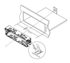
5 Place the supplied rubber cushion over the end of the mounting bolt.
