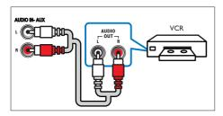
Using an analog cable, connect the AUX connectors on your home theater to the AUDIO OUT connectors on the TV or other device.
