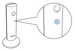
When the handset is placed correctly on the base station, you hear a docking tone (see 'Set the docking tone' on page 21). The LED at the back of the handset flashes once.
