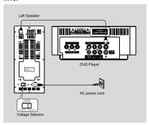
After everything is connected properly, plug in the AC power cord to the power socket.
