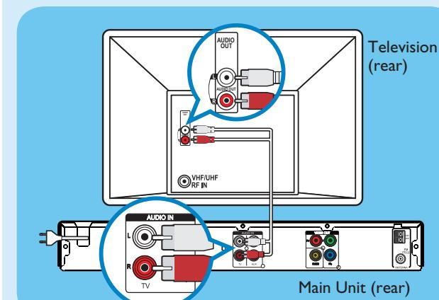
**Note** Press **TV** on the remote control to get the sound output from the speakers system when watching the TV programmes.
