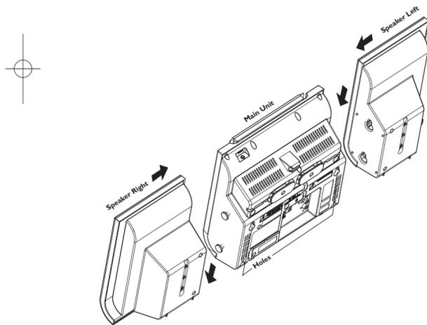
**Use screws to mount the main unit on the wall**
